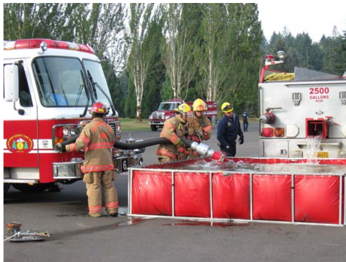
Water tender filling a port-a-tank with water. Crew filling engine.
